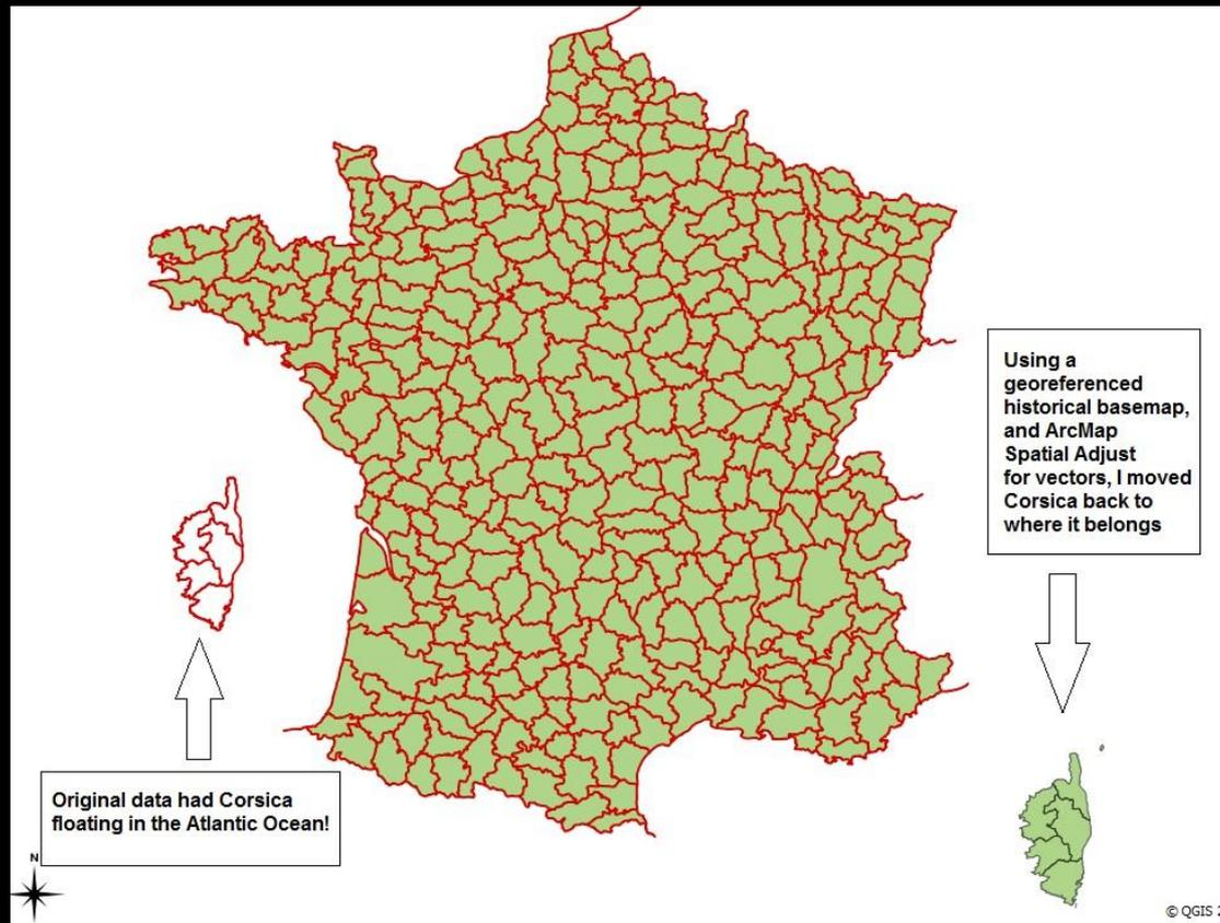
Correcting the position of the Corsica units
